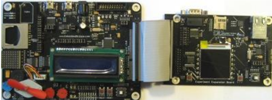
Figure 1 - LPC2148 Education Board with Experiment Expansion Board
