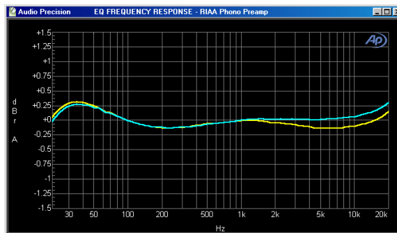
Figure 16. A typical frequency response graph.
