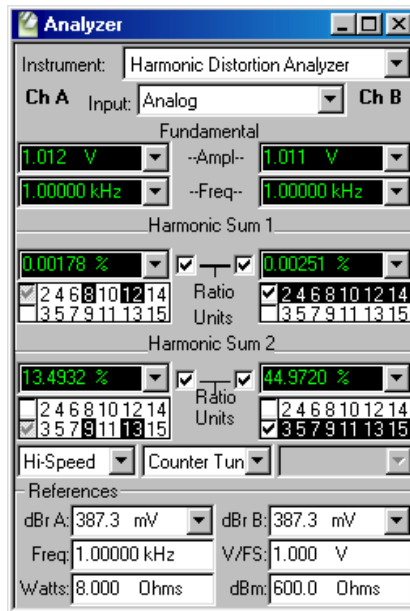
Figure 204. The Harmonic Distortion Analyzer panel.
