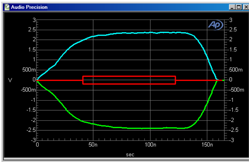
Figure 153. Digital Interface Analyzer eye pattern (48 kHz rate).
