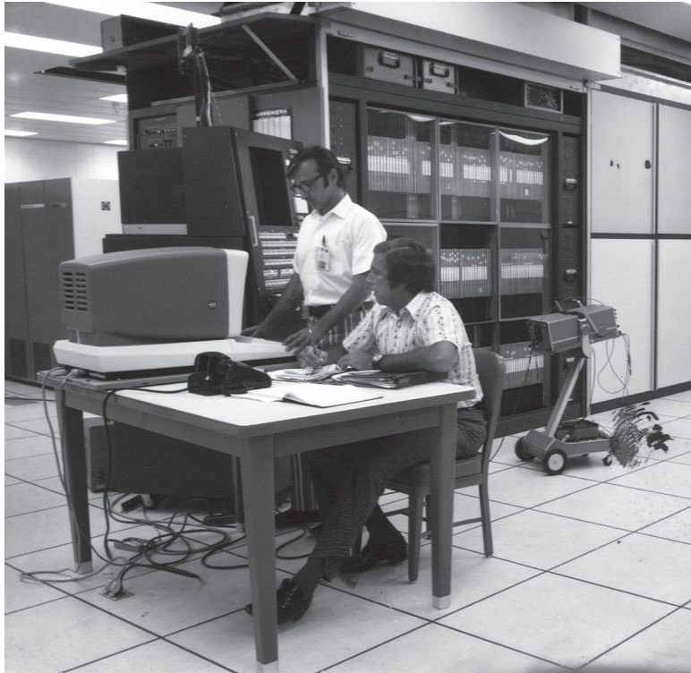
FIGURE 6.15.1 The Illiac IV control unit followed by its 64 processing elements. It was perhaps the most infamous of supercomputers. The project started in 1965 and ran its first real application in 1976. The 64 processors used a 13-MHz clock, and their combined main memory size was 1 MB: 64 \times 16 KB. The Illiac IV was the first machine to teach us that software for parallel machines dominates hardware issues. Photo courtesy of NASA Ames Research Center.
