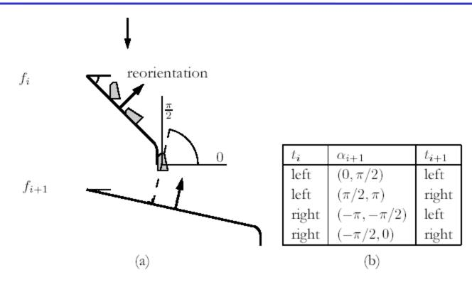
Figure 3.2 (a) For two successive left fences, the reorientation of the push direction lies in the range  $(0, \pi/2)$ . (b) The ranges op possible reorientations of the push direction for all pairs of fence types.
