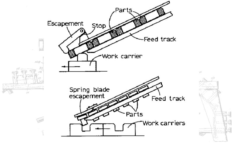
Fig. 5.24 Escapements actuated by the work carrier.
