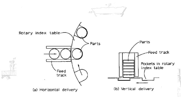
Fig. 5.25 Feeding of parts onto rotary index table.
