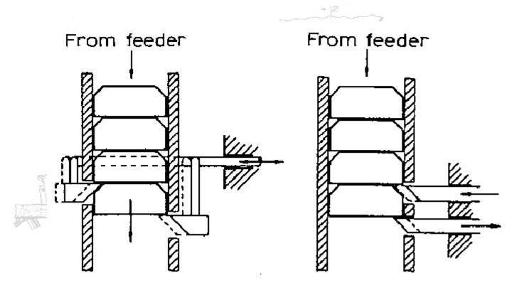
Fig. 5.27 Ratchet escapements operated by linear motion.
