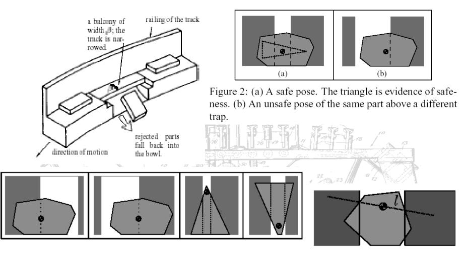
Figure 4: The types of rejected poses.
