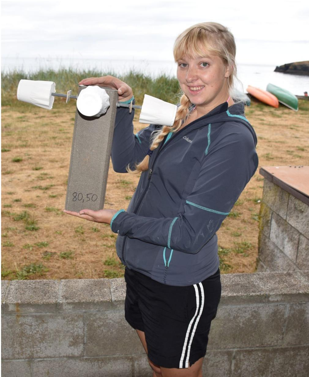
Figure 4. The sleeve holding the clod cards before deployment into the bay.
