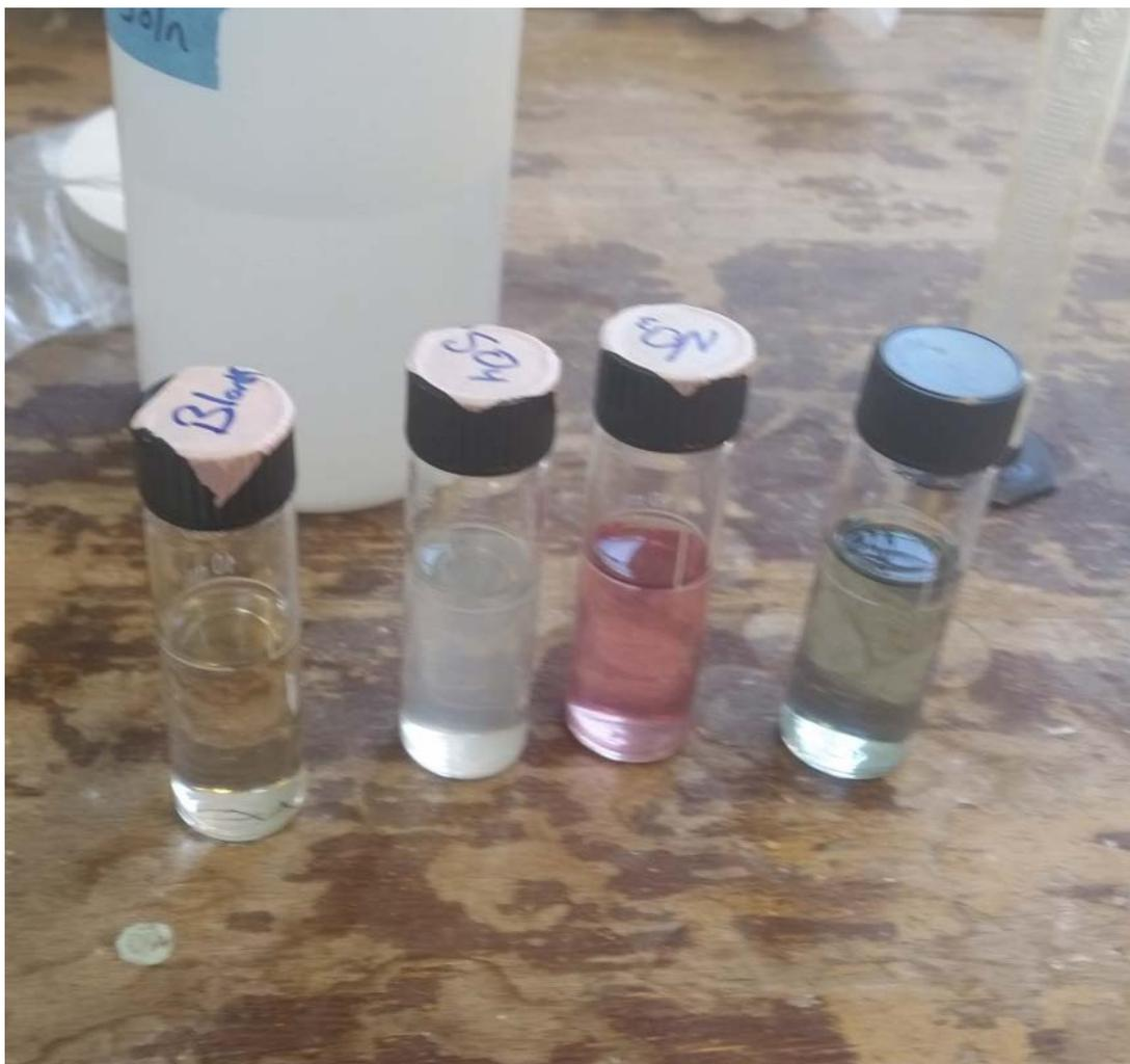
Figure 11. Sediment nutrient tests for sulfate, nitrate, and phosphate. A blank is on the left. These tests were done on the sand/silt portions of three of the sediment samples taken from each site.
