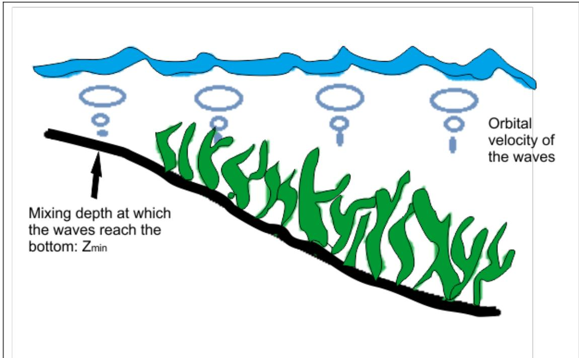
Figure 1. Eelgrass beds can be forced into deeper waters due to exposure to waves. Waves can shift sediment which may affect the ability for the roots to take hold. The zone where waves do not allow eelgrass growth is defined as the depth equivalent to half the wavelength and is the minimum depth of distribution or  $Z_{min}$  (Koch, 2001)
