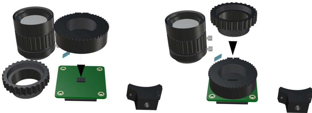
Appendix Figure 23: Reinstallation of lens mount by reattaching hex lock keys to underside of the main circuit board followed by replacement of CS-mount adapter ring for use with wide angle lens (P21).
