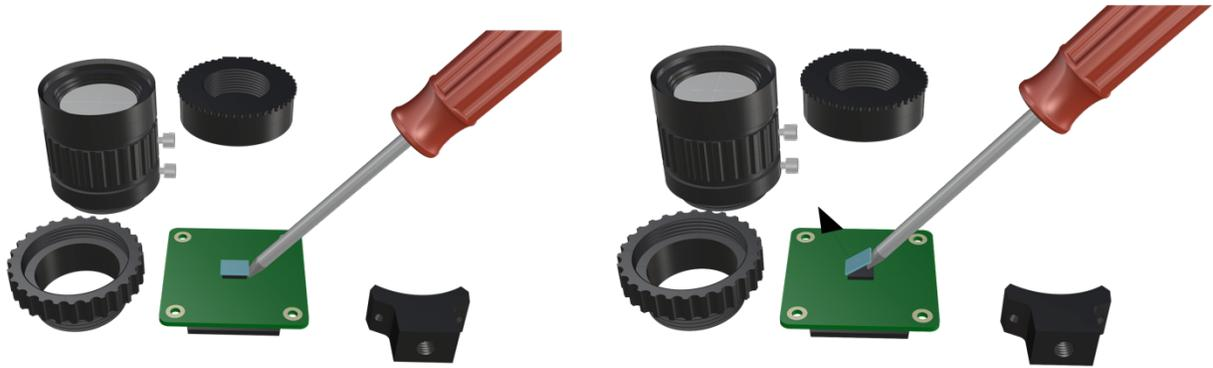
Appendix Figure 22: A flathead screwdriver can be used to remove the FR filter from the Sony IMX477 sensor, removal of the FR filter exposing the sensor.
