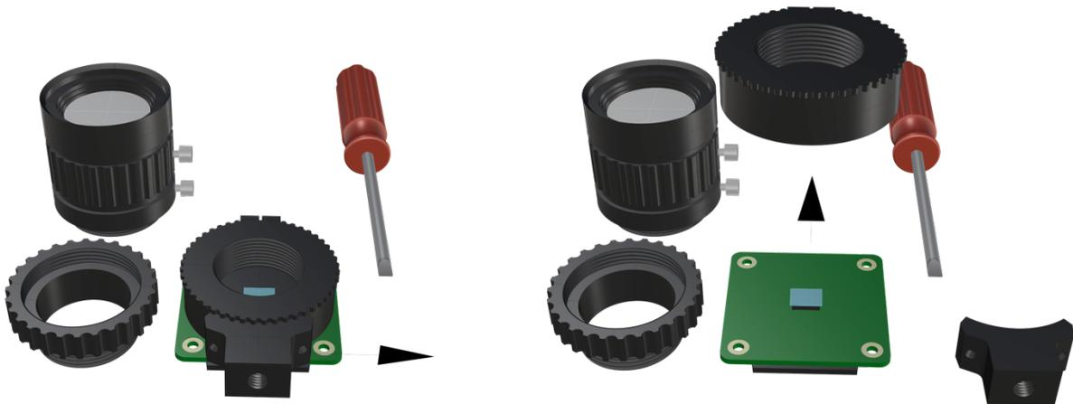
Appendix Figure 21: Permanent removal of integrated 1/4"-20 tripod mount followed by removal of the two 1.5 mm hex lock keys on the underside of the main circuit board to remove the lens mount and expose the FR filter.
