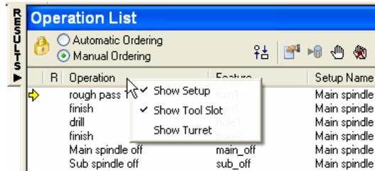
4. Check the *Show Setup* option. This will display a new column in the Operation List called *Setup Name*. This column lets you know which spindle will be used to run an operation.
