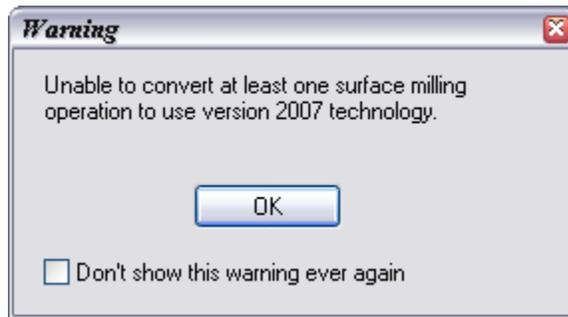
Each incompatible operation is labeled so that it will use the version 2006 machining library to compute tool-paths. This label is visible in the operation list right-click menu (see next section). All compatible operations in all the surface milling features will automatically use the new machining library. All new features and operations created in FeatureMILL3D 2007 will only use the new machining library. A detailed list of the incompatibilities is included later in this document.
