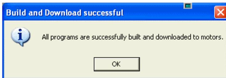
Now, to run the program, click on the 'Run' button. This will result in the downloaded programs running in all the motors. By default, the generated programs run the homing routine initially. This behavior can be changed using the SMP Programming Environment since BCD programs are basically SLA OS generated SMP programs.
