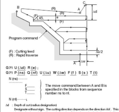
Designate without sign. The outfing direction depends on the direction AA'. This designation is modal and is not changed until the other value is designated. Also this value can be specified by the parameter (No. 5132), and the parameter is changed by the program command.
